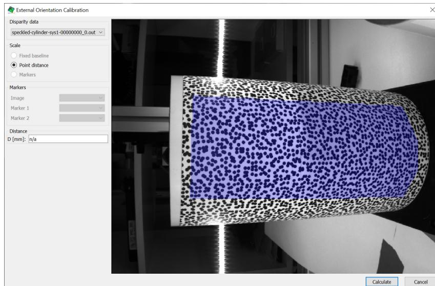
Since we will be using marker information for the baseline, click the **Markers** radio button. Select the two markers and enter the known distance between them in mm in the **Distance** line editor. This is the resultant distance in 3D space between the two markers irrespective of the curvature/shape of the object.
