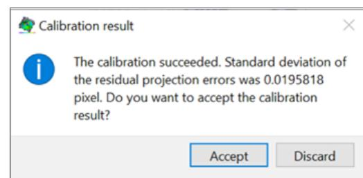
The score should be very low (less than 0.1). Click **Accept** to complete system calibration and save the project.
