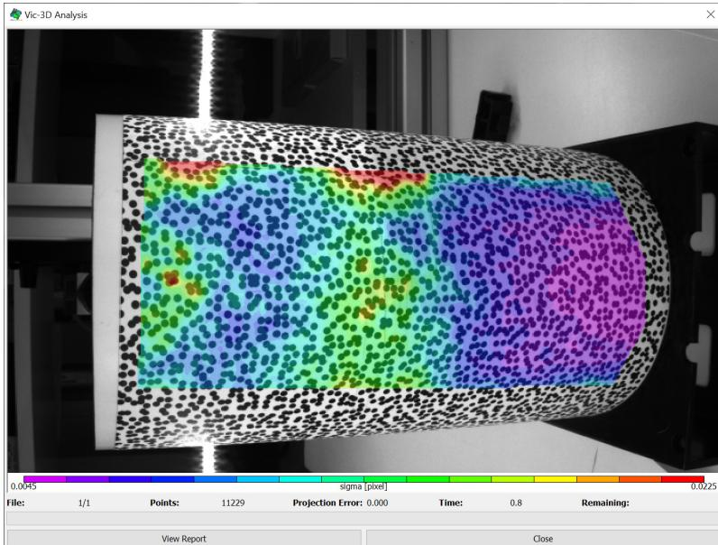
To complete the extrinsic calibration, a very accurate distance in the field must be known. This is best accomplished using the existing markers. Click the *Marker Editor Workspace* button in the main toolbar to enter the Marker workspace:
