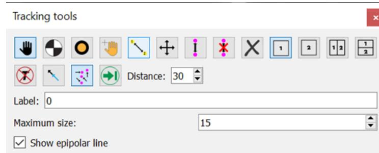
Then, for at least three visible markers (more may be used for error reduction), click the marker in the image view. A marker overlay should snap to the displayed marker and match the shape and size; if it does not appear or appears incorrect, you may need to adjust the *Maximum* size to be equal to or greater than the size of the marker, in pixels.
