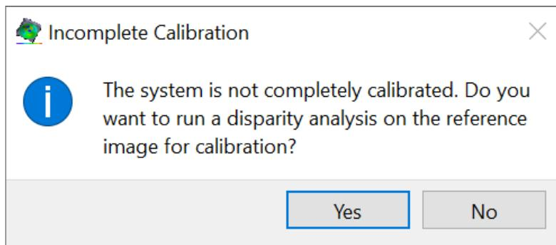
After running the analysis, the disparity result will be shown. If no points were analyzed or if part of the AOI is missing, it may be necessary to add an initial guess (using the AOI tools) and retry.
