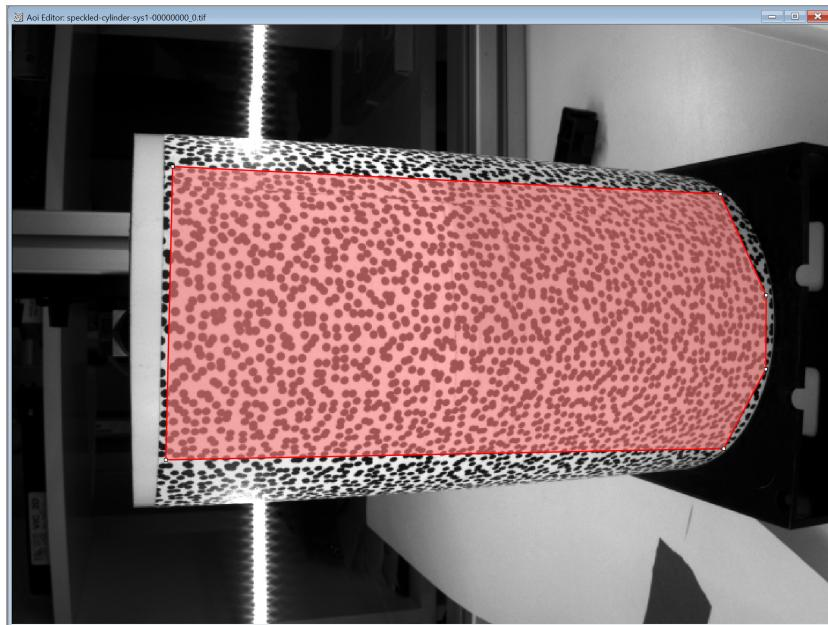
Click **Start Analysis**. You will be warned that a calibration is not present – the resulting analysis will give a *disparity* field but not a 3D result because triangulation is impossible at this stage.
