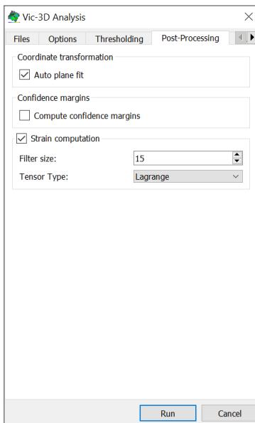
This will ensure that our results are in the real Cartesian system we established earlier and not a new and inconsistent auto plane fit system.
