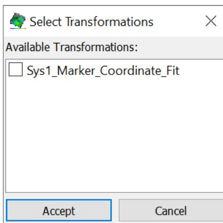
Select the transform from the step above and click **Accept**. The internal camera locations should now match their actual coordinates in real 3D space, so that future correlation with this calibration will give results in a consistent and real Cartesian coordinate system. With this done, save the project with a meaningful name (sys1-final-cal or etc.).
