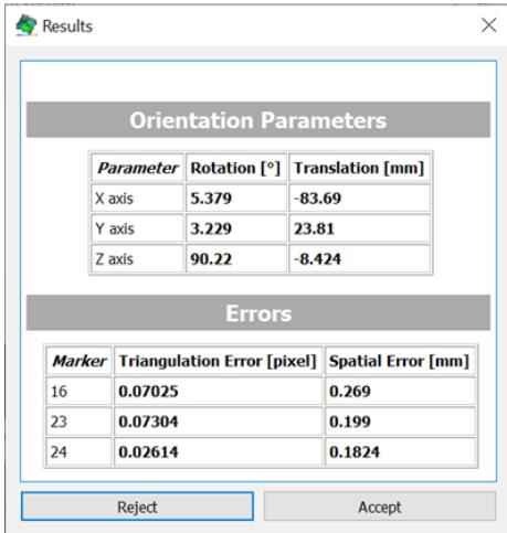
Click **Yes**, then **Calculate**. A result display will appear. Both the Triangulation and Spatial error should be low (<<1); if any are particularly high, the marker may have been extracted incorrectly, or a marker may be named incorrectly, or a physical coordinate measured incorrectly.
