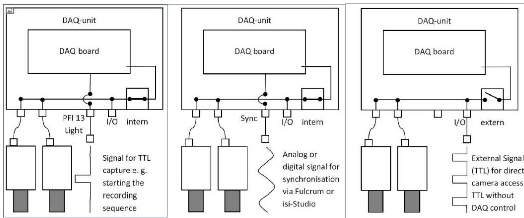
**Standard Hardware trigger mode / TTL trigger mode (left):** With this setup, the “TTL Capture” method in VIC-Snap can be used. This setup also provides the standard hardware triggering of the cameras, -for this case no TTL signal has to be connected to the PFI 13 / Light connector. In VIC-Snap the hardware trigger mode has to be selected.
