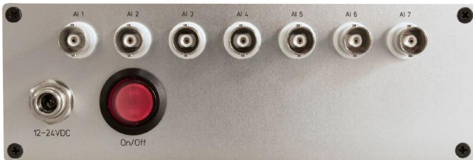
–The connectors "AI 1" to "AI 7" are differential analog inputs, the range is +/-10V
