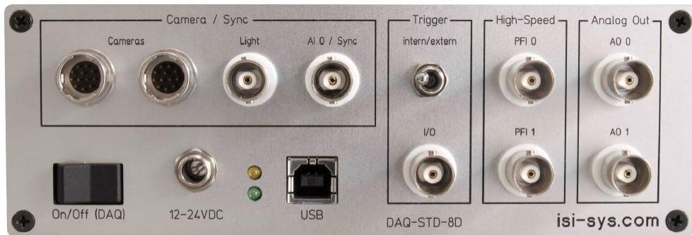
–2x 12 pin Hirose connector (upper left area) for connection of up to two cameras (camera power supply and camera trigger are transmitted).
