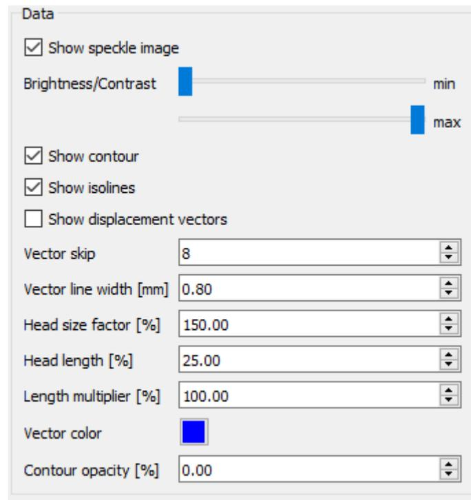
Figure 15.34: Data tool for 2D plot of triangulated data.
