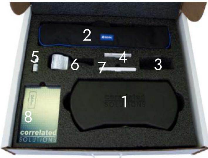
1. The stereo vision measurement head containing two cameras for stereo imaging, a light to illuminate specimen, and connections required to power the cameras and output data
