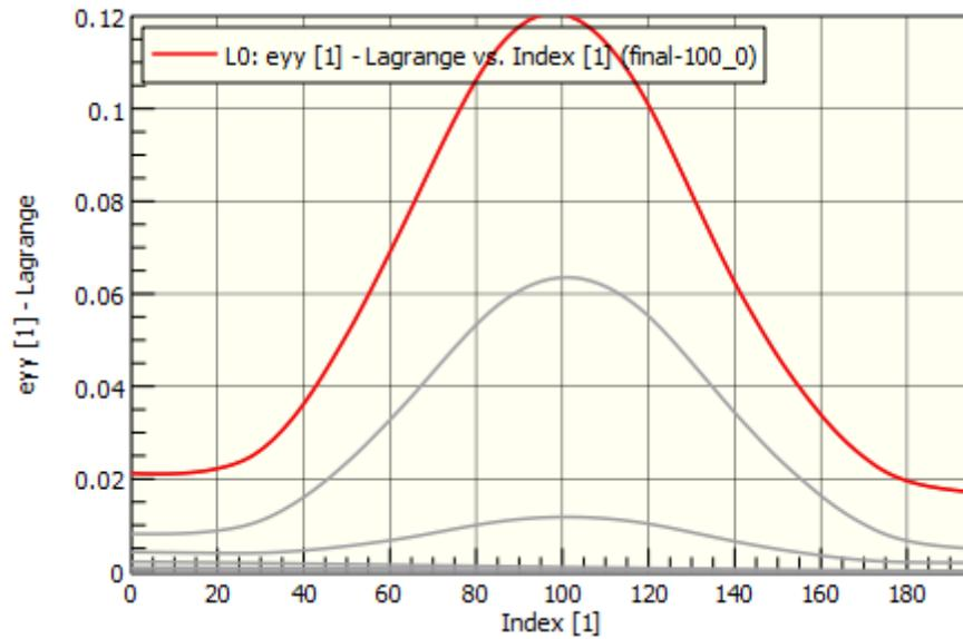
Here the current file (the .out file selected in Current Data) is red and the other lines that are shown are grey. In the Extraction Tools, the Settings will allow you to format the graph with the Styles Tab. The Line slices Tab allows for the user to select which files are shown in this line plot as well as additional format options for the lines.
