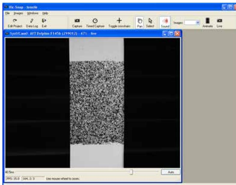
When the camera is at the same height and lateral position as the specimen, and the specimen is centered in view, it follows that the optical axis is correctly normal to the specimen.
