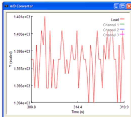
This data is saved in the CSV log file associated with the project. This file will have the same name as the project prefix and for each image set, contains the image count, the filenames, the exact times, the unscaled analog data, and the scaled analog data.
