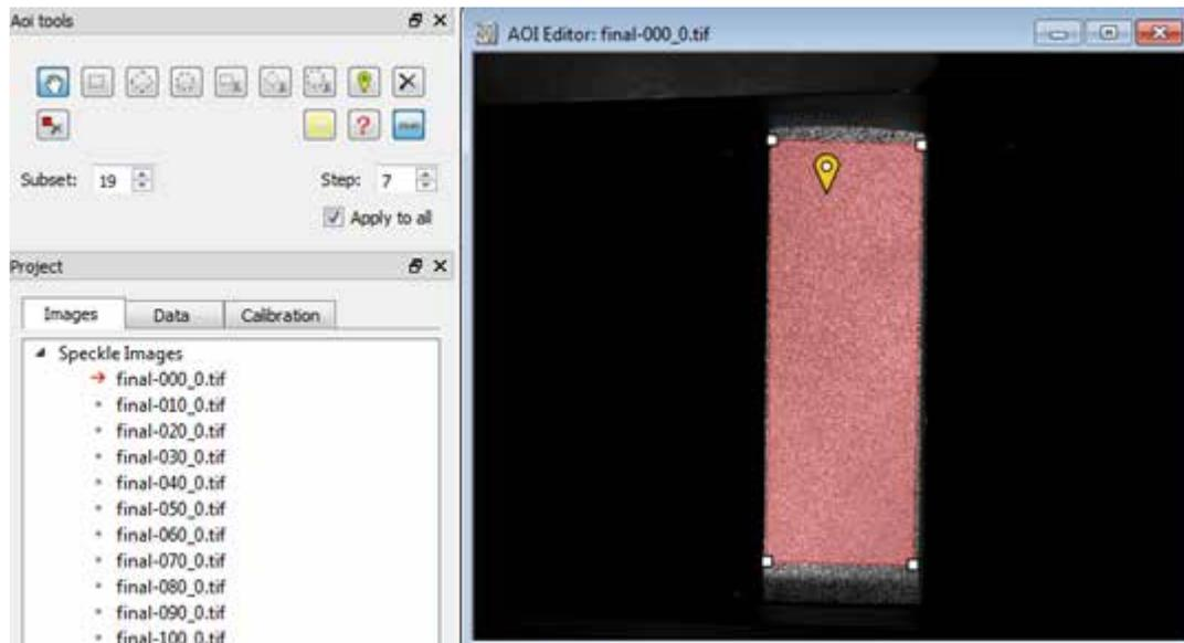
In order to select a good initial guess point (also called a seed point), an area with good definition and contrast should be selected in order to allow a successful automatic guess. The seed point subset should look similar in the reference and deformed subsets. Also a seed point with low strain should be selected. The seed point should be in an area of low motion; i.e., in a tensile test, this would be the side of the specimen nearest the fixed grip.
