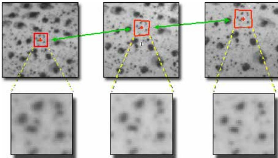
In DIC, a small subset of the image is tracked as the specimen moves and deforms. To perform the tracking, the subset is shifted until the pattern in the deformed image matches the pattern in the reference image as closely as possible; this match is calculated as the
