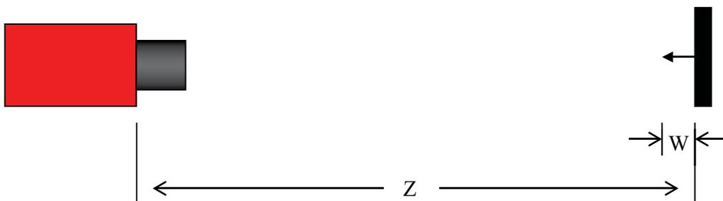
We will minimize the error by reducing  $w$  and increasing  $Z$ . The out-of-plane motion can be reduced through testing configuration and procedure. The  $Z$  distance can be increased by selecting a long focal length (e.g., telephoto) lens. In general, select the longest available lens that will allow you place the camera with a line of sight to the specimen and still image the entire area of interest.
