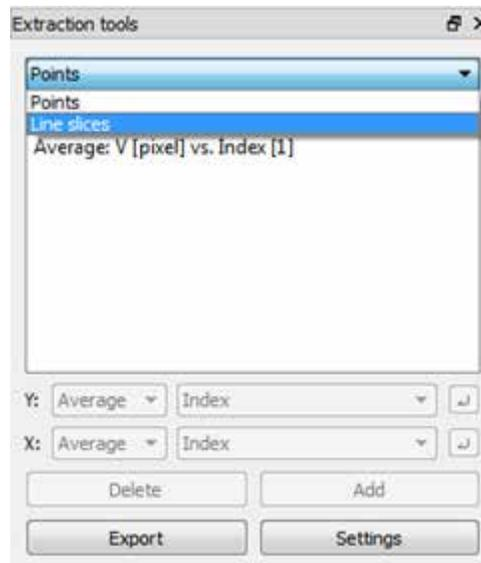
You will now have an extraction plot, with your menu on the left side of the screen, which looks like the image above. Select “Line Slices” from the drop down. Next, select your variables for the X and Y axes and hit the apply button,
