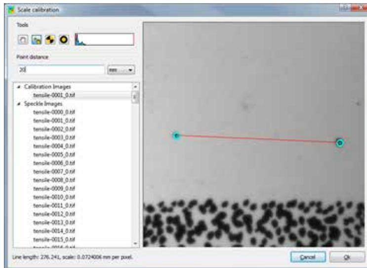
The system is now calibrated, and a scale appears in the **Calibration** tab:
