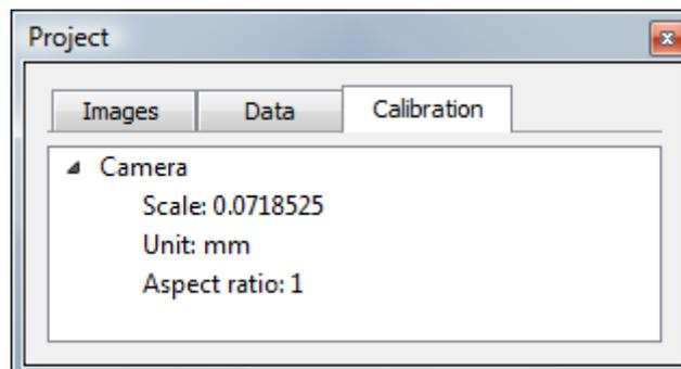
Data analyzed after this point will contain metric dimensions in addition to the pixel units.
