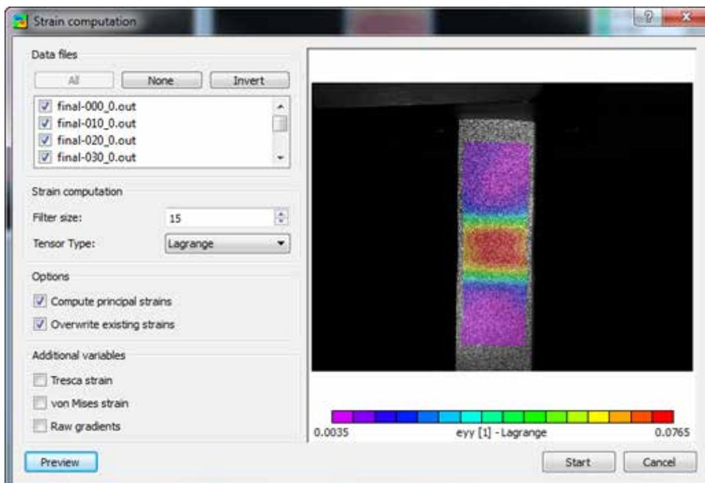
Several options are available but the most commonly used will be the **Filter Size**. It may be necessary to make this value larger to resolve strain when strains are very small. To achieve better spatial resolution and see strain concentrations clearly, use smaller values.
