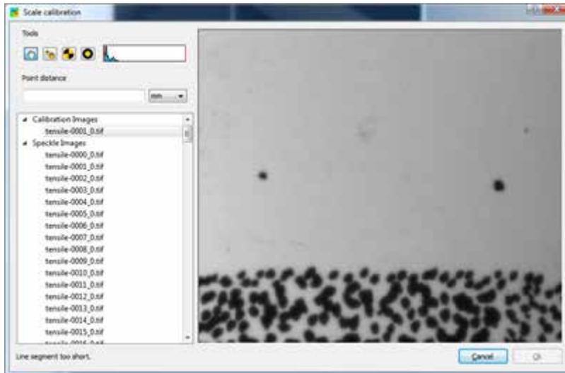
Then, we pick the **Manually select** tool, click on the first point, and drag to the second point. A line appears. We then enter 20 mm in the Point distance box, and click **Ok**.
