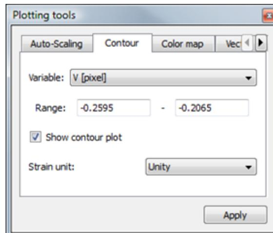
You may either auto-scale the contour limits, or clear the Auto-rescale box and manually enter limits.
