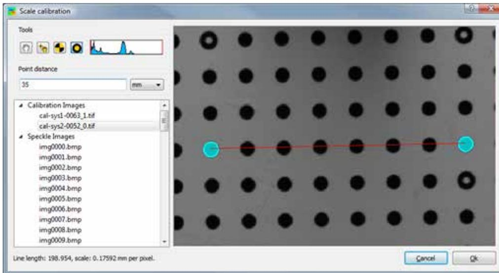
Here, a 5mm pitch grid was used, and there are 7 spaces in between, so the distance is entered as 35mm.
