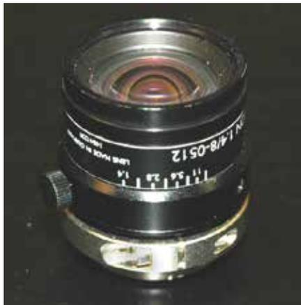
This lens has an aperture ring with a locking knob. To focus, loosen the collar (for this particular lens, a 2mm hex driver is used), and rotate the entire body of the lens. Loosen the lens body (counterclockwise) to focus closer; tighten (clockwise) to focus farther. Tighten the collar when complete.
