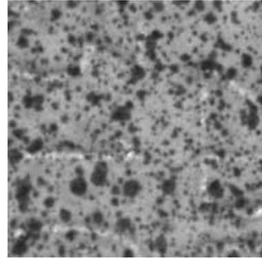
For larger fields, larger blobs must be produced. This can be effected by either modifying the nozzle, or throttling the spray. One effective technique is to place the surface horizontally, and spray over it. If the spray nozzle is barely pushed down, large blobs will come out and fall on the surface; the finer mist will spray over the surface, leaving a good, coarse pattern. The 48" panel below was painted this way.
