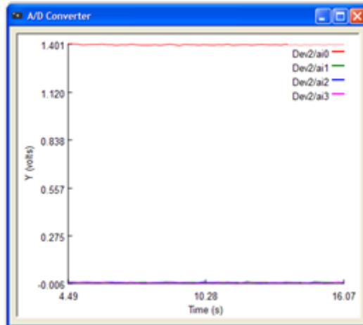
You can double-click on a channel heading to remove it from the display (double-click again to return it). You can also scale and rename these channels; right-click and select **Edit channels**. You can enter a title, range, and multiplication factor for each channel. Selecting the appropriate range will give higher accuracy. To view scaled data, right-click and select **Show scaled**.
