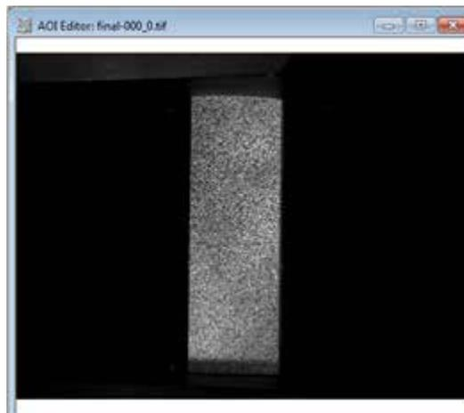
This image is the Reference image; it will be the reference state and all strains and displacements will be relative to this image. By default, the first image in the sequence is the reference; if you would like to select a different image, right-click on the image in the image list at the left, and click **Set reference image**.
