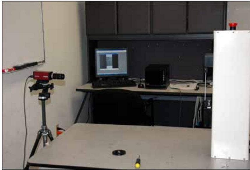
After placing the camera, Vic-Snap is started so that we can preview the image. The height and tilt adjustments on the tripod are used to align the center of the specimen in the center of our view.
