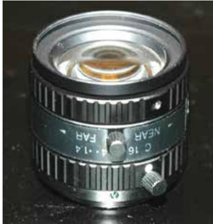
This lens has a focus and aperture ring, each with locking knob. The aperture ring is normally closest to the camera. Loosen the locking knob (if present); make any adjustments; and tighten the lock before calibrating.
