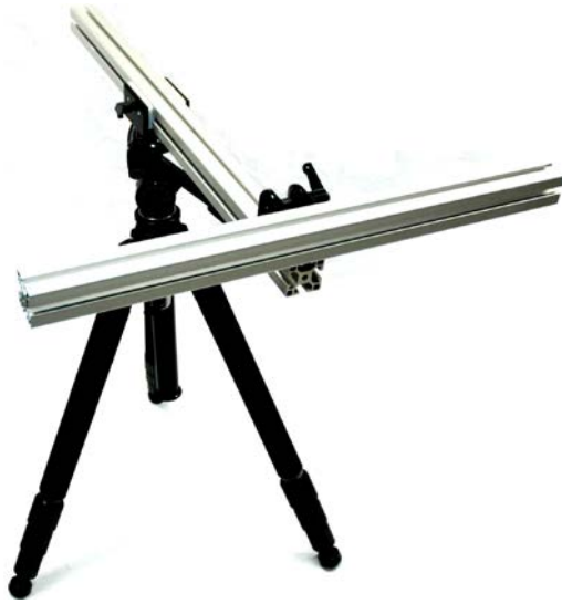
Figure 11. Hinge attaches aluminum extrusions
