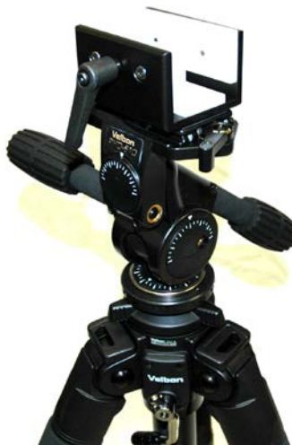
Figure 6. Slide block mounted to tripod 3-axis adjustable head
