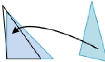
The remaining deformation of the triangle gives us exactly enough data to compute a strain tensor for this triangle. We repeat this for each triangle:
