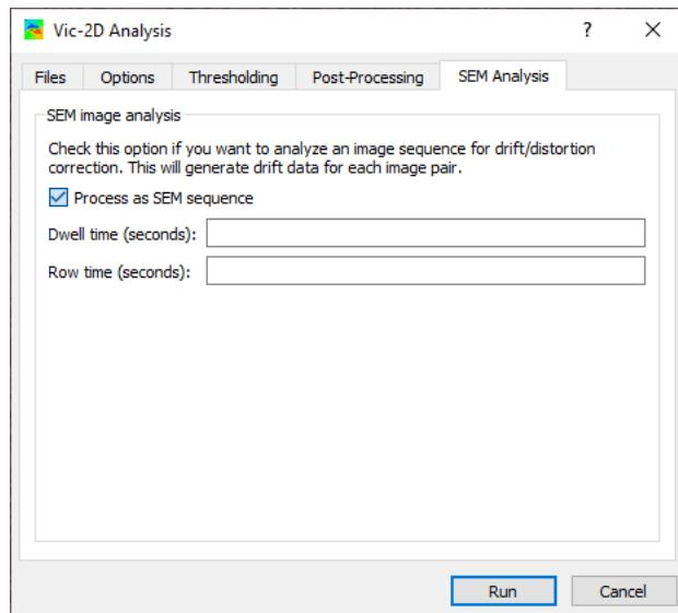
Check the **Process as SEM sequence** box. Enter the dwell time and row time, in seconds:
