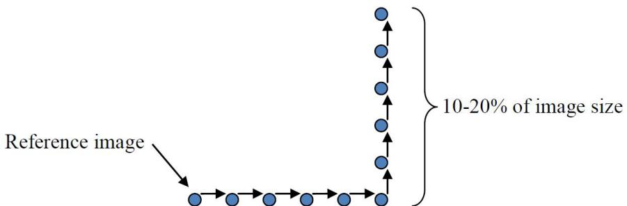
Five motion steps in **each** axis is sufficient for calibration. The **total** motion should be approximately 1/10th to 1/5th of the image size.
