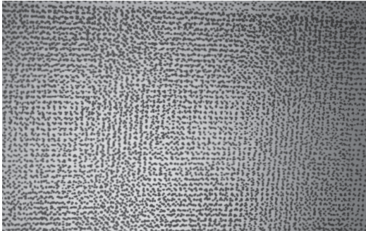
Speckle patterns produced using the Correlated Solutions Speckle Kit.
