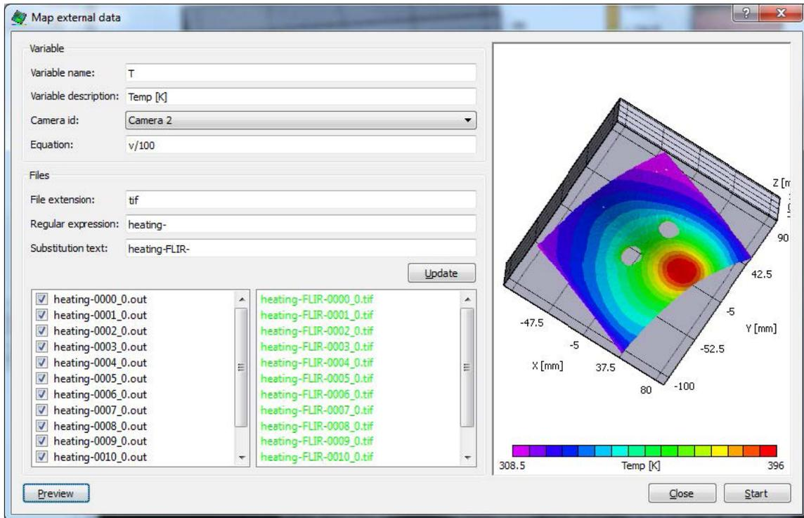
Here, we see that the temperature has been mapped to the object as a new contour variable. The most common issue that you might see at this point is data that is incorrectly mapped:
