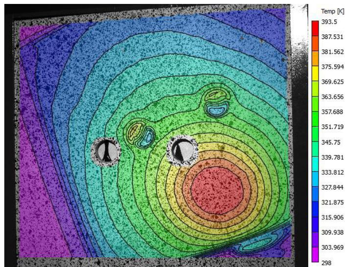
Here, the IR data is skewed relative to the DIC data. In this case, **check the selected coordinate system from the pulldown in the calibration dialogs**. Most likely, a different view was selected for the stereo calibration vs. the external calibration.
