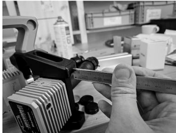
Figure 17: Measuring the camera position against the rail.
