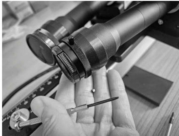
Figure 16: The holder for the polarization filter is secured with a small thumb screw.
