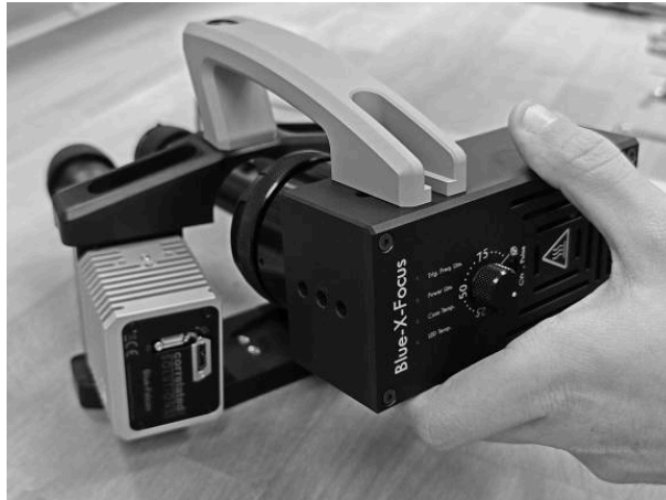
Figure 8: The Blue-X-Focus remounted sideways so the optical path of the lamp matches the optical path of the system.
