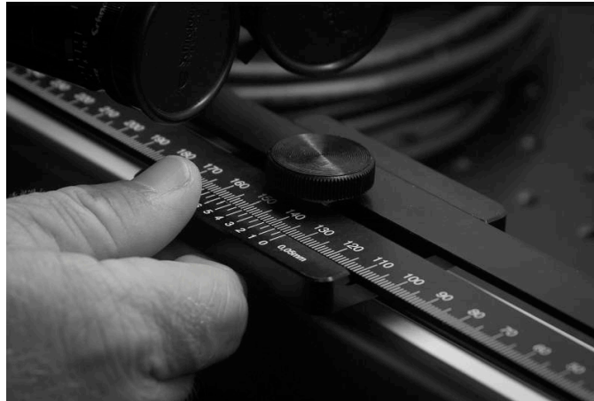
Figure 6: Sliding the gauge to the ruler value for the configuration in use.
