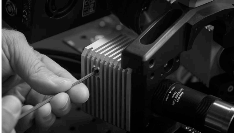
Figure 14: Backing the Scheimpflug angle off to zero with a 3 mm hex key, turning counter-clockwise until it stops.
