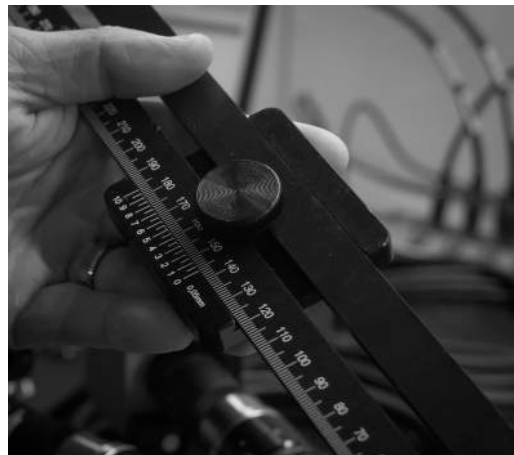
Figure 7: Locking the slider at the ruler value with the knurled screw.
