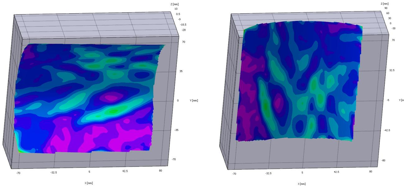
After the transformation, the software will orient the cylinder so that the y axis is axial with the cylinder. This change is shown in the two above images, where the left image is before the transformation and the right image is after the transformation.
