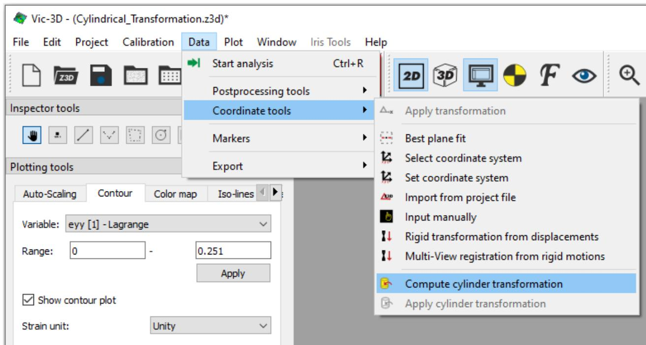
Choose this option, click accept and the software will automatically compute the cylindrical transformation. The software will give how many iterations it took for convergence and give the radius of the cylinder as well as the standard deviation.
