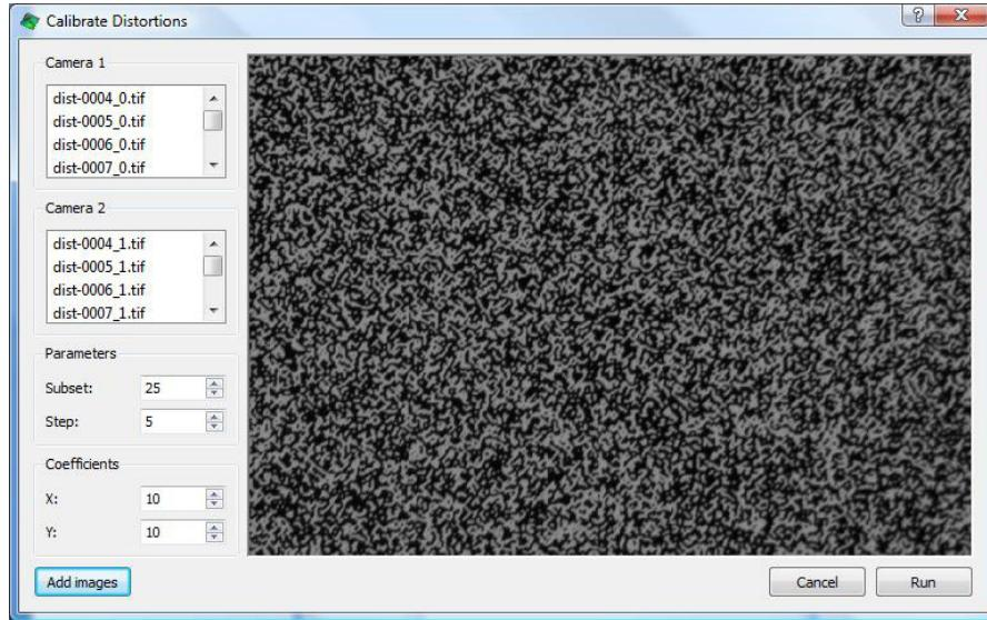
Select a subset size appropriate to the speckle pattern. For the conditions present in a stereomicroscope, the default step size and coefficient values will work well. Click **Run** to start the analysis.
