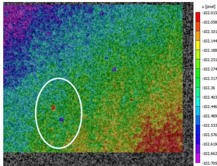
Two obvious erroneous values are circled in white. In this case the cause was dust on the sensor; the dust was cleaned and the analysis was re-run successfully.
