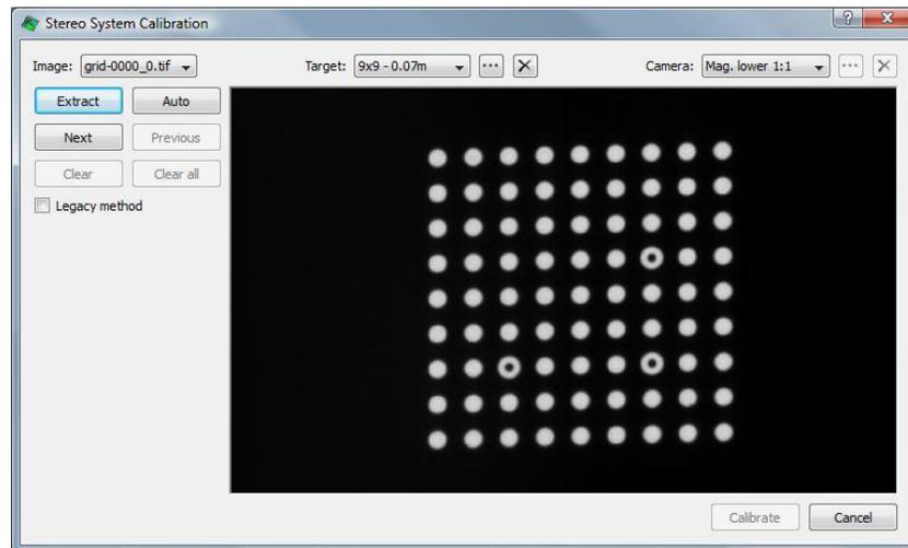
For **Target**, select the grid geometry for the target you used. Here, we've used the 9x9 grid with 0.07mm spacing from the glass 6-in-1 speckle/grid slide.
