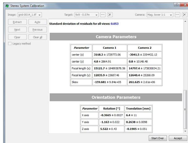
As with normal stereo-calibration, check to see that the standard deviation of residuals for all views is low and represented in blue and not red. Click **Accept** to finish. Save the project once again to store the stereo calibration.
