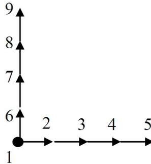
The total motion should be approximately 15% of the field of view, which means each step in the sequence above will be approximately 4% of the field of view. Also, the motions need to be in the exact plane of the pattern itself. It is best to start in the corner of the pattern, as shown, to give the largest final corrected field of view.
